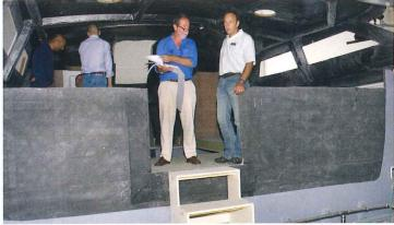
A classic deck line belies the yacht's high-tech construction, with hull and deck built in pre-preg carbon to keep the displacement at 60 tonnes. The interior structure, from the longitudinal stingers to the bulkheads, is also carbon. and she will carry a carbon mast from King with conventional rod rigging. Each bulkhead is trimmed and topped with a flange (right) to ensure a perfect seal with the deck once the interior elements have been fitted
