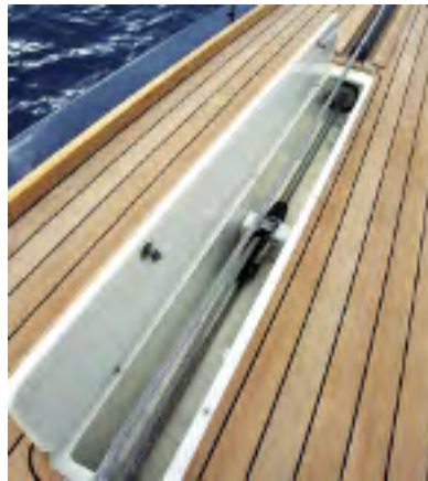
Details: carbon guides the anchor, whilst genoa trim is oil-pressure-assisted.
