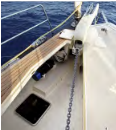
Details: carbon guides the anchor, whilst genoa trim is oil-pressure-assisted.
