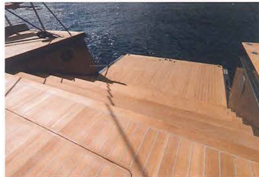
Left: clean lines: note the tight headsail sheeting angle thanks to a three-line barber system. Below: a key feature on deck is the stern platform, designed by Nauta Yachts as a way to welcome guests in a grand manner. The teak-laid after deck hinges over to become the bathing platform, revealing a shallow staircase
