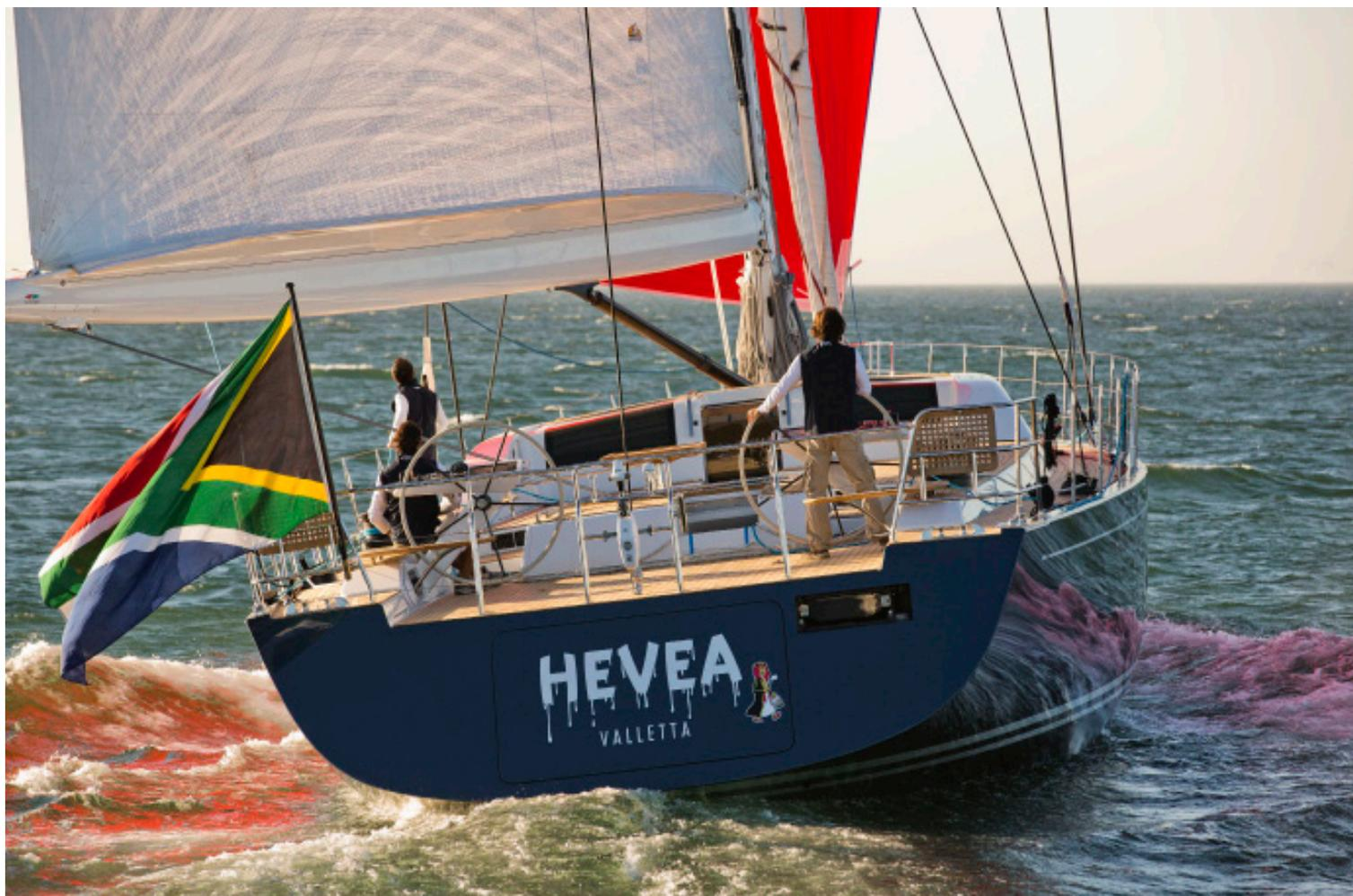
**THE NEW HULL BY FARR HAS ALLOWED A 17 PERCENT INCREASE IN INTERIOR VOLUME COMPARED TO THE SW 100**
